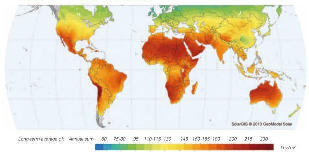
$\text{KLy} = 4,19 \, \text{kJ/cm2} = 11,63 \, \text{kWh/m2}$ hour of sunshine =  $33 - 77 \, \text{Ly}$  (average  $45 \, \text{Ly}$ )
